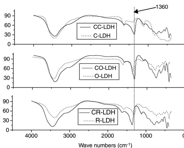
Fig. 5 – Infrared analysis of LDHs before and after CO<sub>2</sub> capture.
