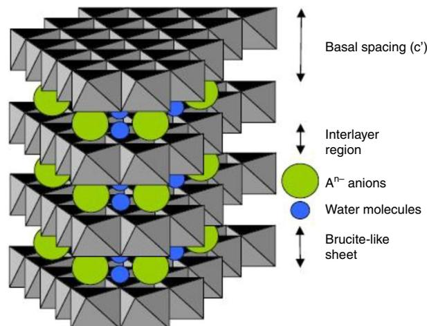
Fig. 1 – Schematic diagram of LDHs structure.
