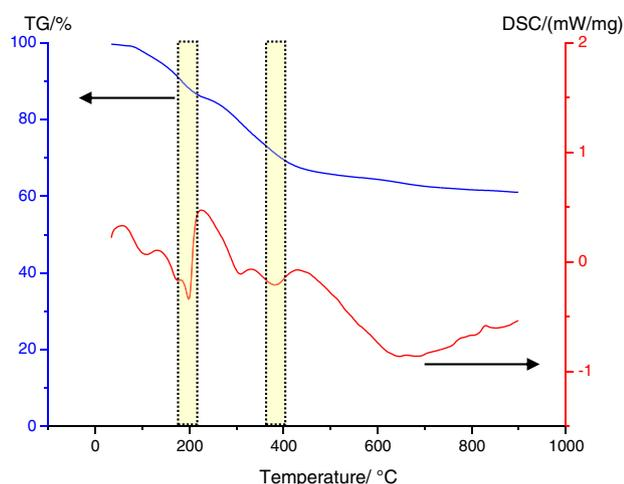
Fig. 3 – TG/DSC of Mg–Al–CO<sub>3</sub> type hydrotalcite.
