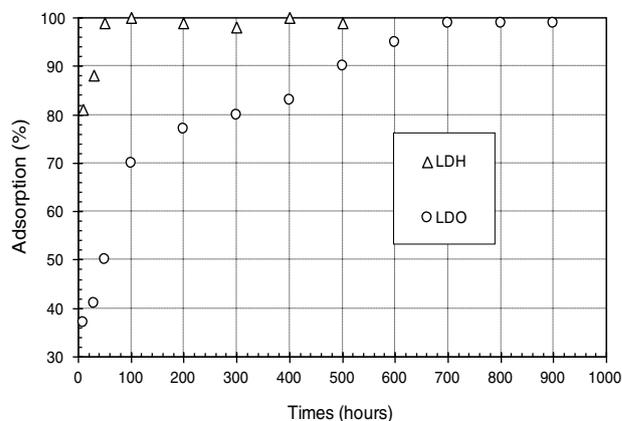
**Fig. 6 – Time dependence of adsorption of  $\text{CO}_3^{2-}$  by LDHs and LDOs.**
