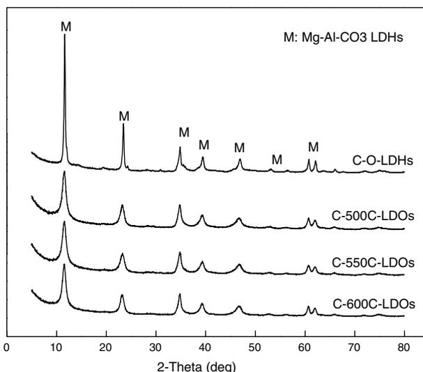
Fig. 2 – XRD patterns analyses of different types of LDHs.
