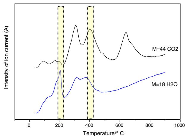
Fig. 4 – Mass spectrometry of Mg–Al–CO<sub>3</sub> type hydrotalcite.
