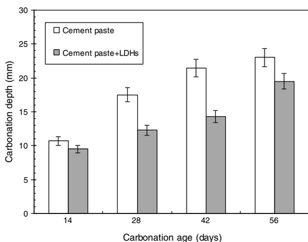
**Fig. 7 – Carbonation depth of cement paste mixtures containing LDHs at different ages.**
